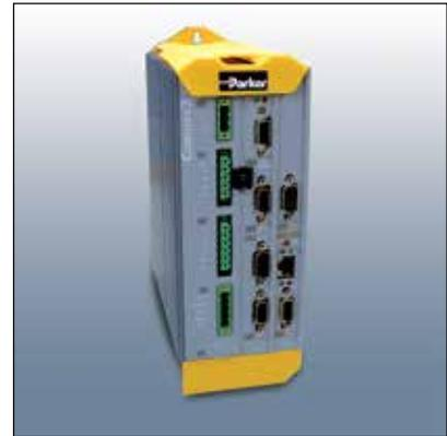
With its high performance and modular design, the Compax3 family of industrial servo drives and drive/controllers offers a new level of servo performance and flexibility. Available in single- or multi-axis configurations, with numerous expansion options, all models are rated for 120-480 VAC input, continuous current output from 2.5 A (rms) to 155 A (rms), and are CE (EMC & LVD) and UL compliant.
